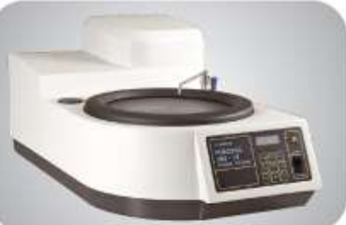
FORCIPOL 300-1V, Variable speed unit for 300mm. wheel application
