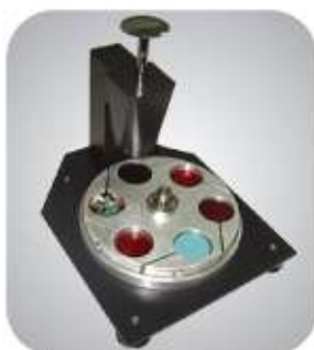
Levomat Specimen Loading Fixture to level specimens for central force specimen holders.
